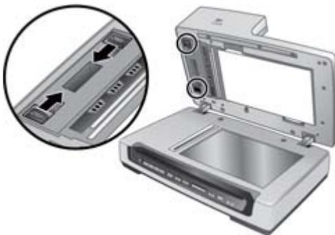
4. Locate the clear scan window inside the ADF and clean it with the ADF cleaning cloth.
