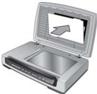
12. Place the film templates in the scanner storage slot.
