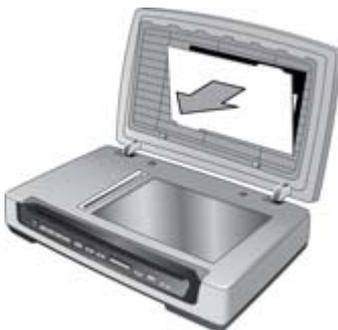
4. Place the negatives into the appropriate template using the icons on the template to guide your film placement.
