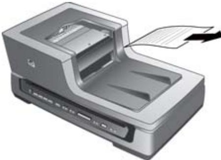
3. If the jammed page still cannot be removed, lift the lid to its fully open position, loosen the jammed page from the roller on the underside of the lid, and then gently pull the page out of the ADF.
