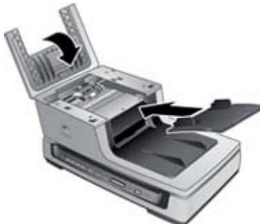
5. Put the input tray on the ADF. Reload the unscanned pages in the ADF input tray.
