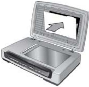
11. Place the film templates in the scanner storage slot.
