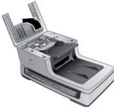
2. Lift the green lever to raise the feed-roller assembly to the vertical position.
