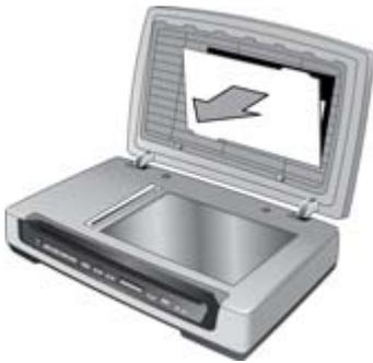
4. Place positives in the appropriate template, using the icons on the template to guide your film placement.
