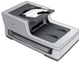
2. Adjust the paper guides to center the stack. Pull out the input tray extension for longer paper sizes.
